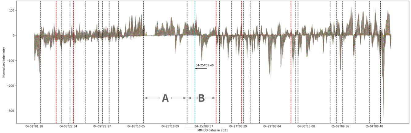
Figure 1: Stacked normalized telemetry view of BOBCAT-1. Parameters: time windows of 25 minutes, stride of 10 minutes and distance threshold of 50% to trigger breakpoints. Black and red dashed bars are BETSI breakpoints; the red dashed bars are the strongest behaviour changes. The cyan dashed bar is the operators' feedback on the critical event where spacecraft entered safe mode and de-tumbling was deactivated. Periods A and B mark periods around the closest breakpoint to the reported anomaly.
